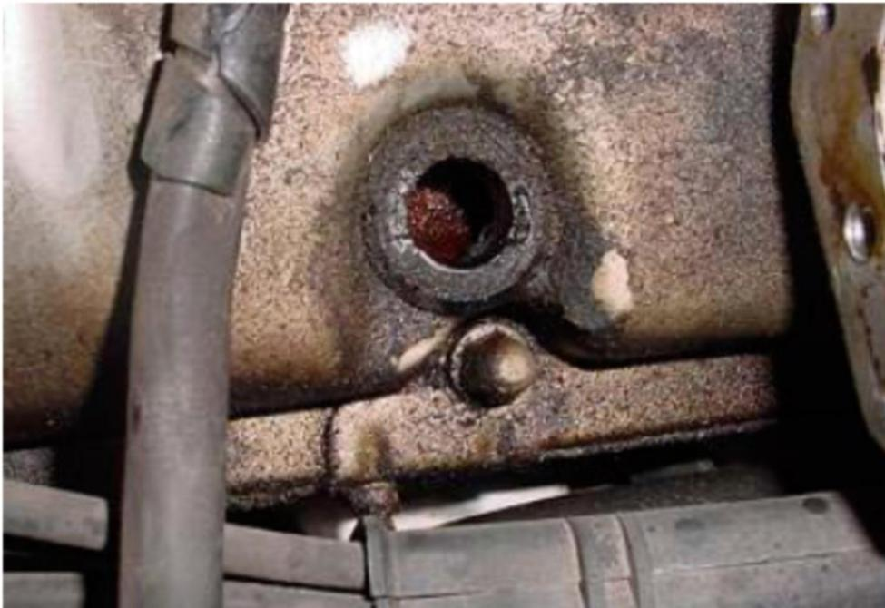
**BOTTOM:** This is the left PCV valve rubber seal/grommet in the valve cover after the PCV valve has been removed.
