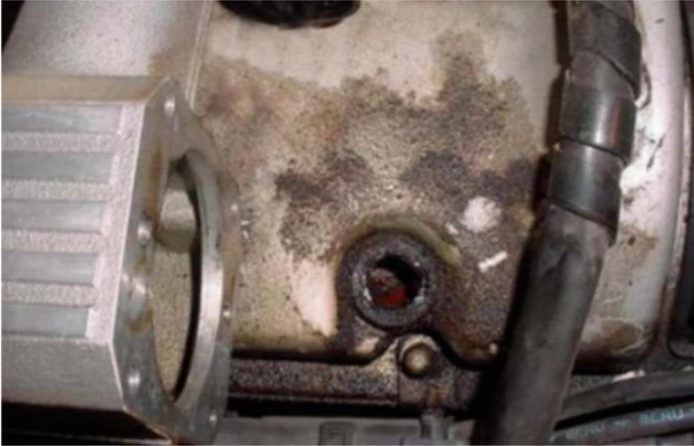
Remove the PCV valves by pulling them up and out of the rubber seals/grommets. Both of these seals will most likely need to be replaced on your engine as they typically have hardened and leak.
